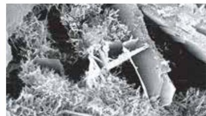
Test piece of PPS waterproof admixture-applied cement (5,000 magnifications)
