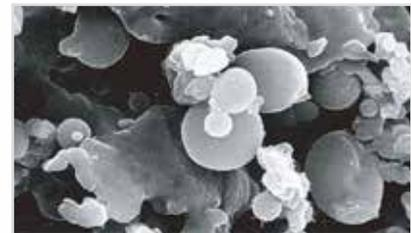
Inner Texture of PPS-applied Cement Paste (4,000 magnifications)
