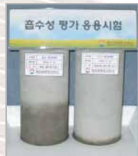
The floor being in contact with water for 10 days after having been dried at 105°C in an oven for 3 days and cooled in a drying chamber for 1 day
